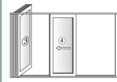
Each panel then swings open and stacks parallel providing full use of the opening
