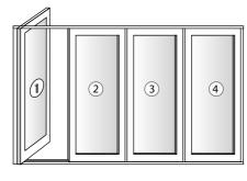
The first panel is hinged and can be on either side of the opening.
